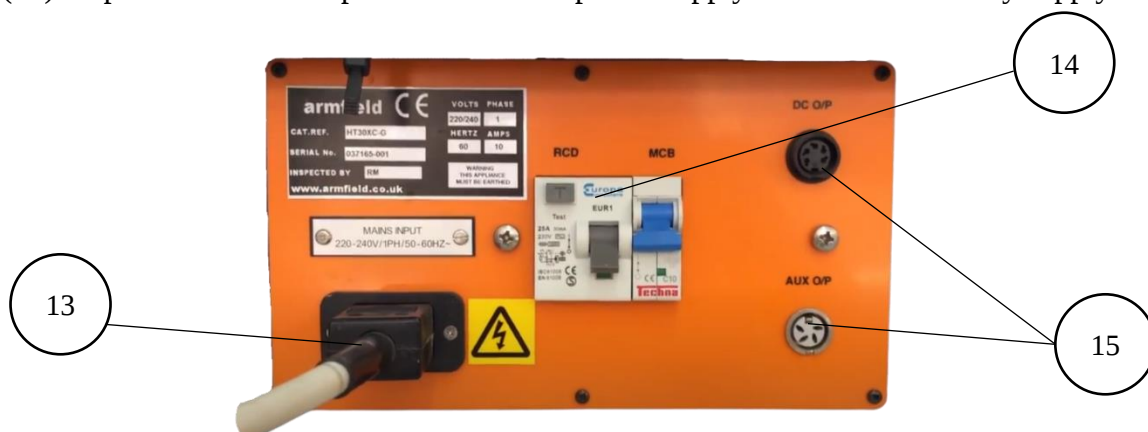
Figure 5. Panel located at the rear of the plinth of the HT30XC Heat Exchanger Service Unit
