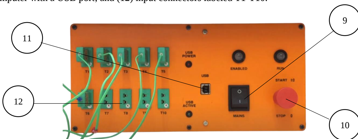
Figure 4. Front Panel of the HT30XC Heat Exchanger Service Unit
