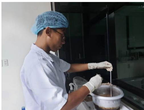
Figure 4.2 Alkali treatment of dried seaweed
